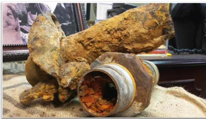
City of Rockdale Water Pipes - Mineral Deposits
