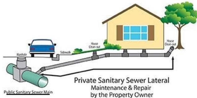
3. Does the city offer assistance? The city Water/Wastewater Department offers help when a service line is blocked. If a service has a properly installed service line cleanout at or near their property line the city will utilize a high pressure jetter to attempt to clear any blockage. This help is contingent on equipment and personnel being available.
